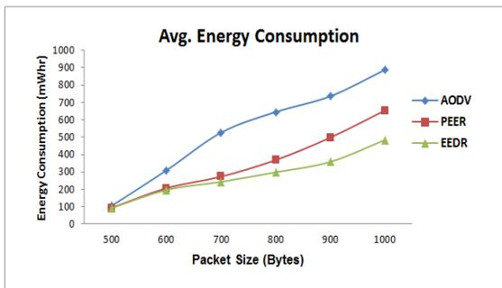
Figure-9: Average Energy consumption v/s packet size (Bytes)
