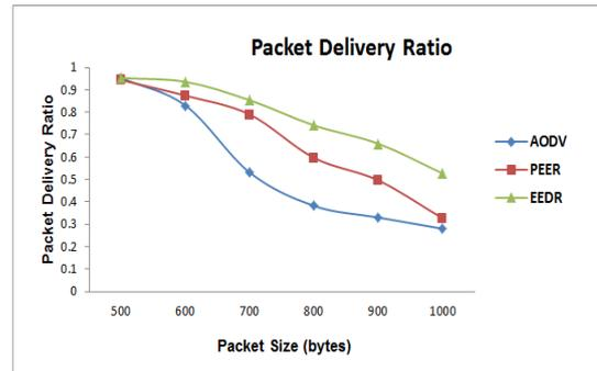
Figure-7: Packet delivery ratio v/s packet size (Bytes)
