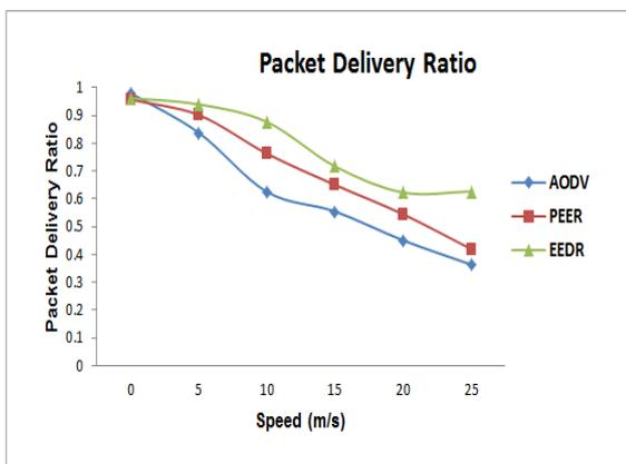
Figure-3: Packet delivery ratio v/s node mobility speed(m/s)
