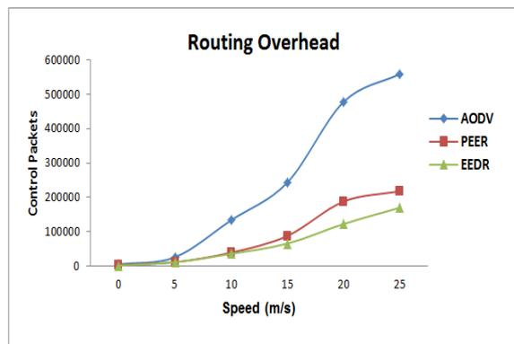
Figure-4: Routing overhead v/s node mobility speed (m/s)
