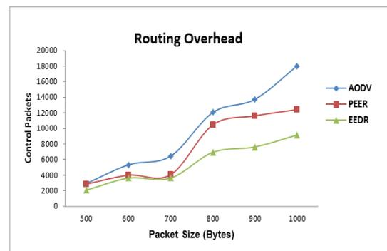
Figure-8: Routing overhead v/s packet size (Bytes)
